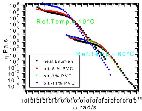
Figure 2: Master curves of  $\eta$  for bitumen and bitumen blends as a function of  $\omega$  at  $T_0=10$  and  $60^\circ\text{C}$
