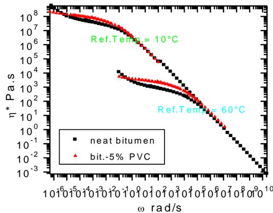
Figure 5: Master curves of  $\eta^*$  for bitumen and bitumen blends as a function of  $\omega$  at  $T_0=10$  and  $60^\circ\text{C}$
