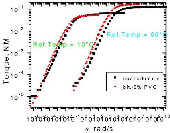
Figure 1: Master curves of torque for bitumen and bitumen blends as a function of  $\omega$  at  $T_0=10$  and  $60$
