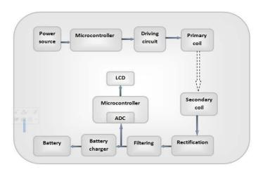
Fig. 1. Block diagram of WPT system.
