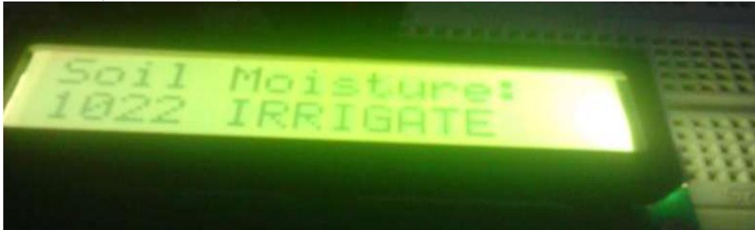
**Figure 11: LCD of sensor value >800**
