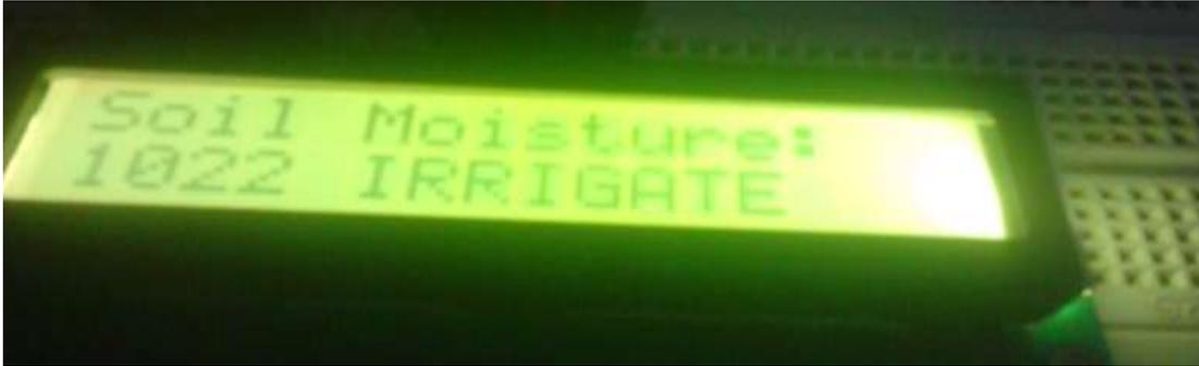
**Figure 11: LCD of sensor value >800**
