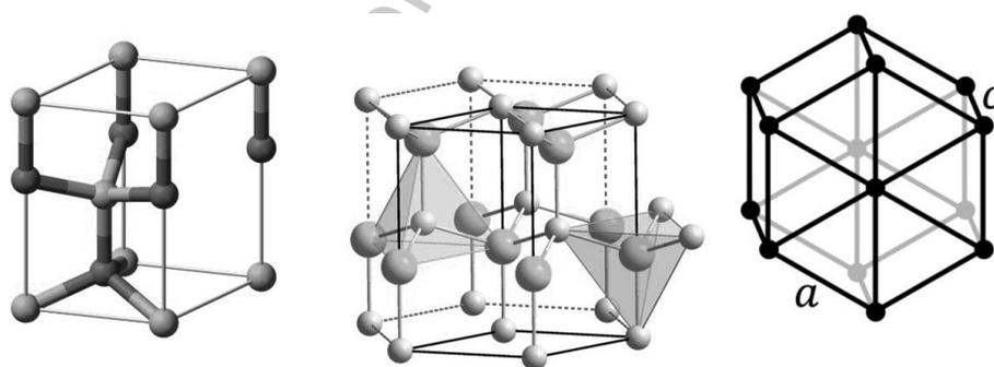
*Figure 4.2* Schematic representation of the principle of unit cells in X-ray crystallography with the example of the Wurtzite crystal structure (a mineral structure). Unit cells are the smallest repeating unit (left) from which to infer the general structural dimensions of the crystal (middle) and its geometric arrangement of the crystal (right). Unit cells act as an index. Images taken from Benjah-bmm27, 2007 (left); Solid State, 2008 (middle); Mayer, 2007 (right).
