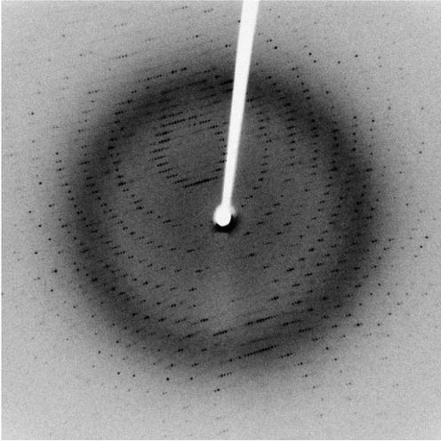
Figure 4.3 X-ray diffraction pattern (image from Dahl, 2006). Concentrated rings of spots are the result of the diffracted X-rays, which are emitted from the crystal and collected on an imaging plate. Spots indicate electron clouds.
