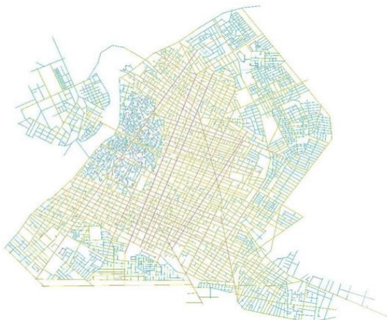
Fig. 14. Integration (R3) distribution of Dezful urban grid. The blue path enjoys better conditions regarding the space configuration and this means that this path should have been popular amongst sightseers
