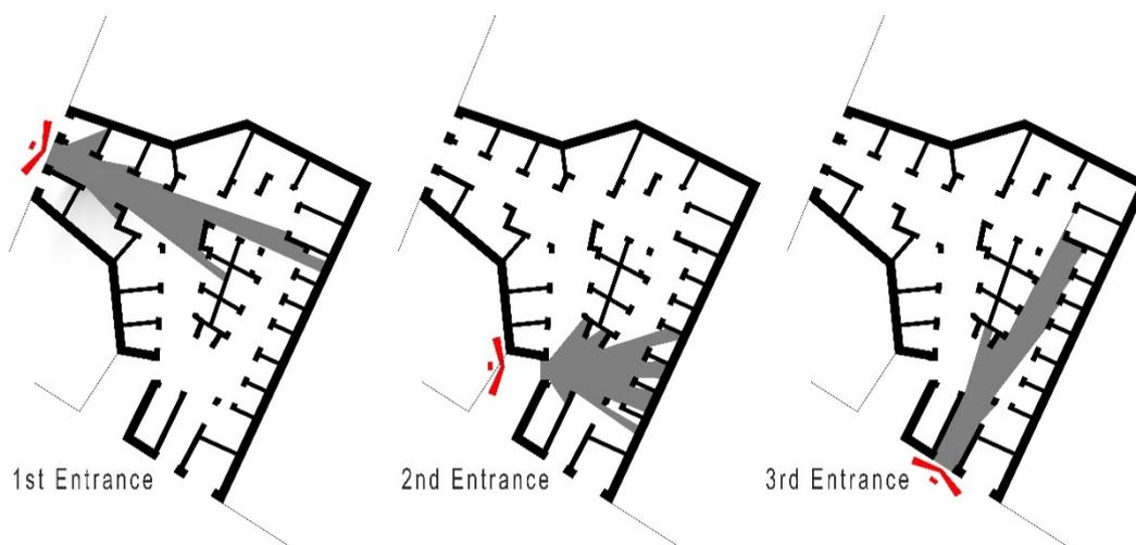
Figure 6. Visibility polygons of different entrances of “Makine Aardi Dastpacheh”.
