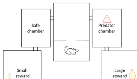
Fig. 7 Environment Choice Test (Bračić et al., under review). The test apparatus consists of five interconnected chambers. On each side, there are cue chambers where predator cues (“predator chamber”) or clean bedding (“safe chamber”) are introduced. During the test, mice need to traverse one of these chambers to finally reach a reward: by going through the predator chamber, they could claim a large reward and through a safe chamber, a small reward
