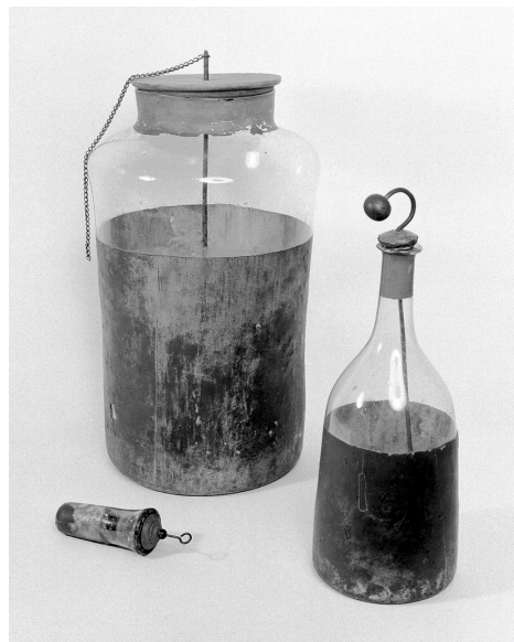
Figure 2. Left: Apparatus used by Galvani - three Leyden jars. Credit: Wellcome Collection. Attribution 4.0 International (CC BY 4.0).
