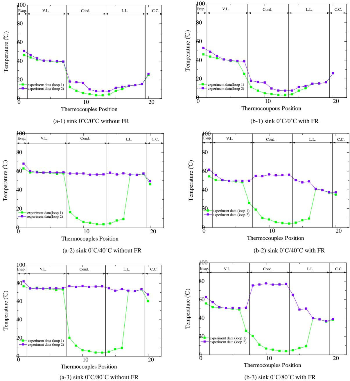
**Figure 6.** The temperature of all parts of MLHP in steady state.
