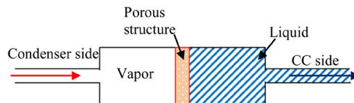
**Figure 2.** The schematic of flow regulator.
