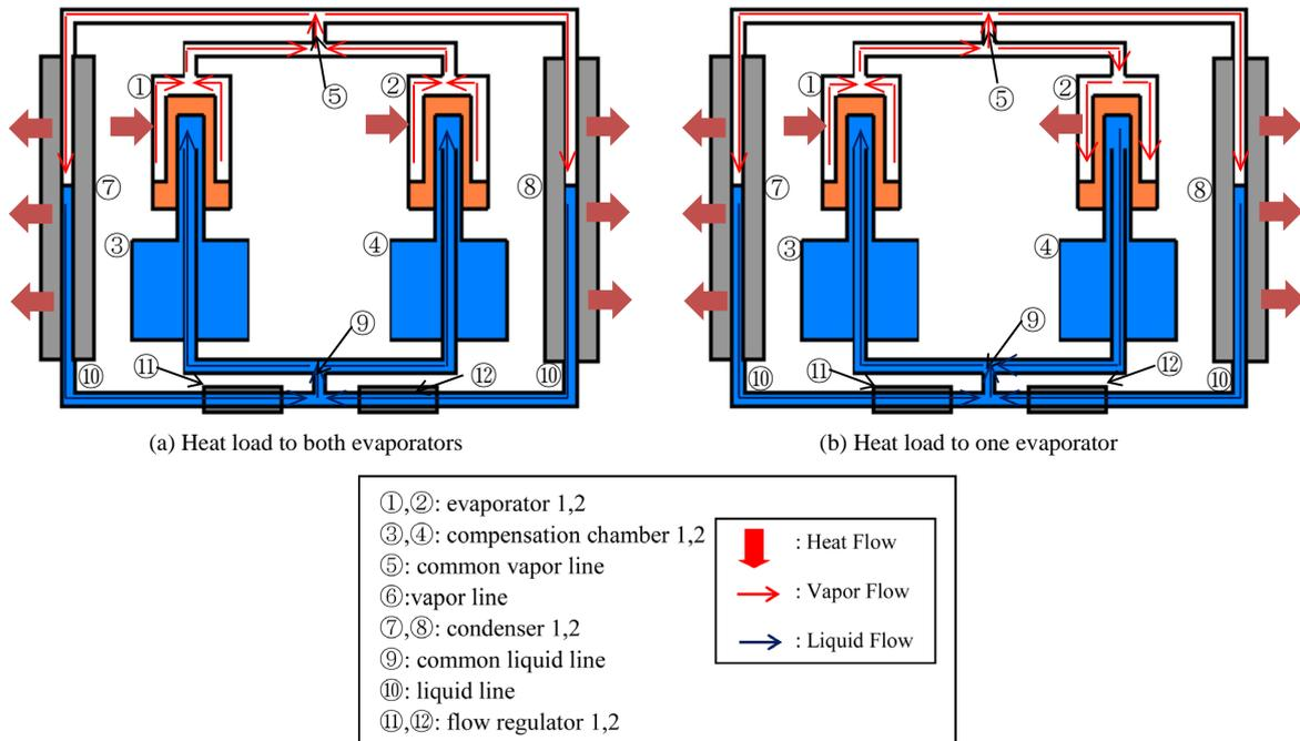
**Figure 1.** Schematic of a MLHP.
