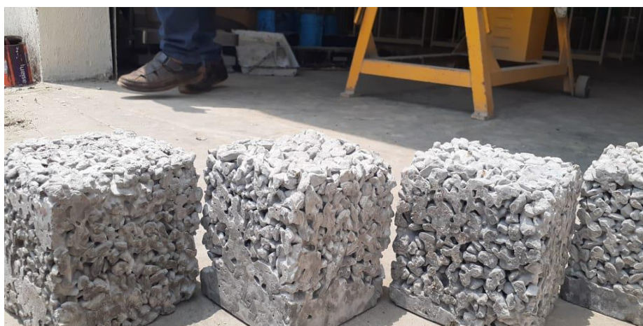
Fig. 5: Accumulation of Cement Paste at bottom
