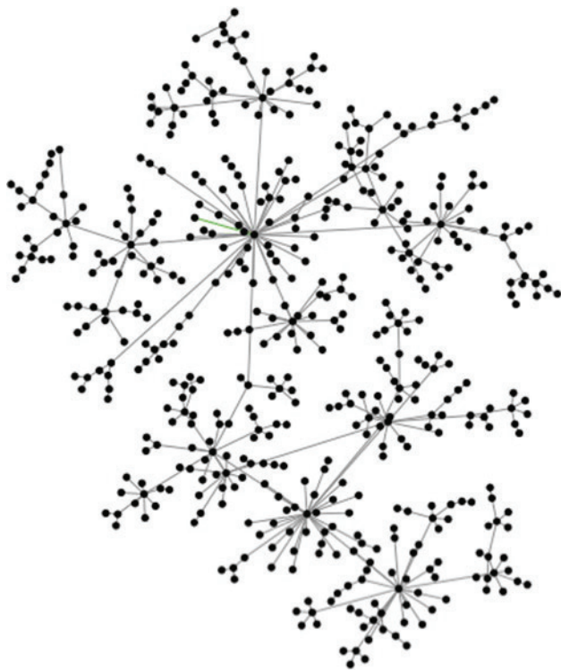
Fig. 1 An example of a network with 500 nodes with links distributed as a power law
