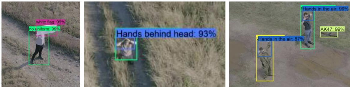
Figure 3. Highly-magnified examples of classifier detecting and classification as part of a video stream: (i) a person without uniform with a white flag, (ii) non-uniformed person with hands behind their head, and (iii) two persons each with hands in the air, which are separated from an AK47 gun.
