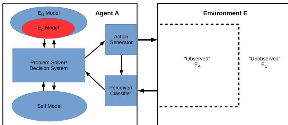
**Figure 1.** General set-up for the Frame Problem (FP): a finite agent *A* interacts with an environment *E*. The agent has perception and action modules and a problem solver. The problem solver has access to two generative models, one of the environment and the other a “self” model of its own problem-solving capabilities. The environment is divided into a part  $E_A$  to which *A* has observational access and a remainder  $E_U$  to which *A* does not have observational access.
