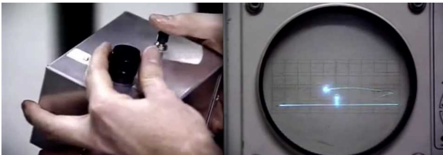
Higinbotham, William: Tennis for Two, 1958, Systron Donner Analog Computer, Germanium transistors, oscillograph (diameter: 5 inches), 2 boxes with turning knobs and press keys. Screenshots from YouTube .
