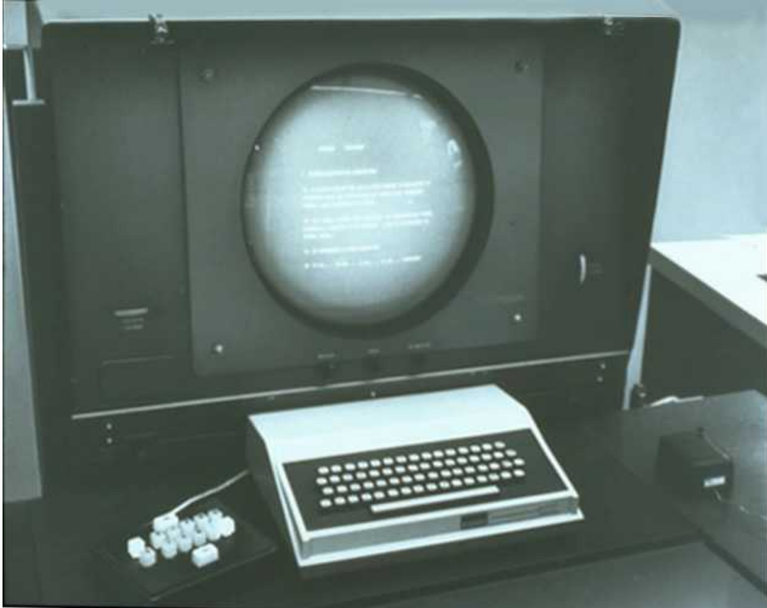
Augmentation Research Center, Stanford Research Institute, Menlo Park: terminal with monitor, keyboard, keyset and mouse, ca. 1964.
