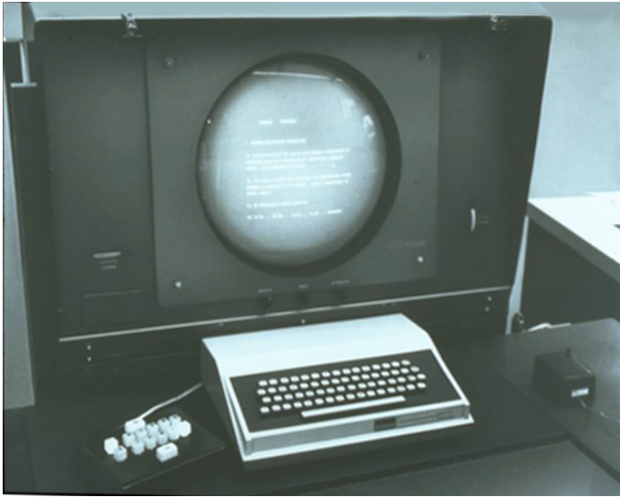
Augmentation Research Center, Stanford Research Institute, Menlo Park: terminal with monitor, manual, keyset and mouse, ca. 1964.
