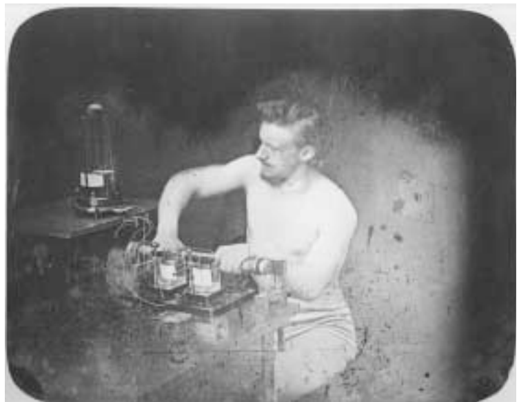
Figure 5 An early daguerreotype of Emil du Bois-Reymond demonstrating the existence of the 'voluntary tetanic current', or nervous signal, by tensing his right arm. His fingers dangle in saline deriving vessels. Wire leads run to the galvanometer on the table to his right. The galvanometer needle, which is suspended from the thread in the glass bell, swings at the moment of muscular effort. Du Bois-Reymond is unclothed to prevent static interference.
