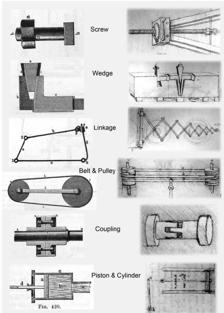
Figure 47: Moon's comparison of kinematic elements in machine design from the books of Franz Reuleaux (on the left) and drawings of Leonardo da Vinci from the *Codex Madrid I* (on the right).
