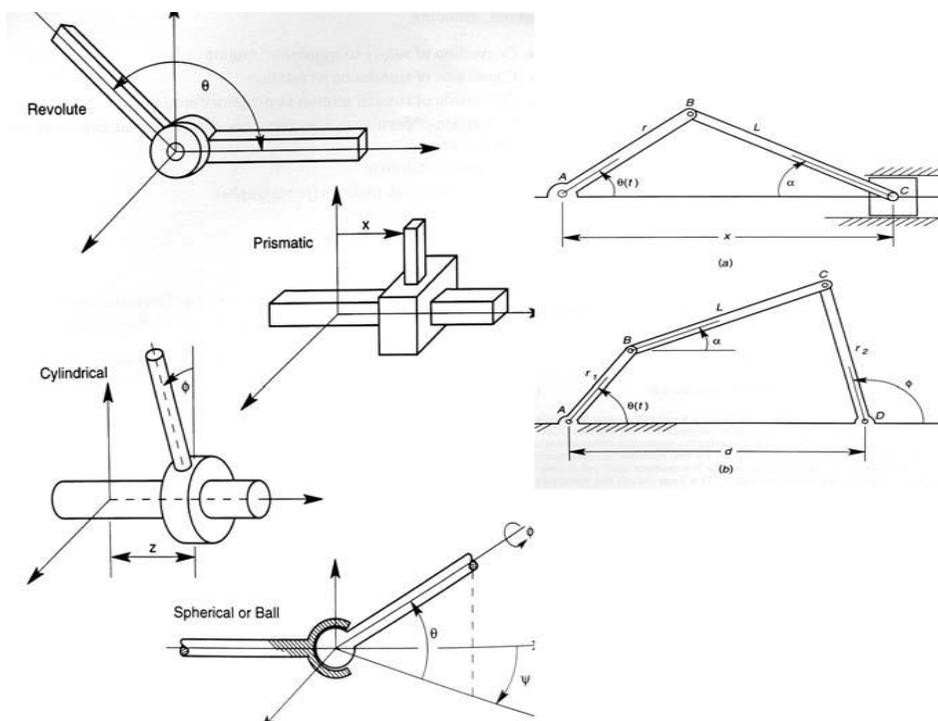
Figure 34: *Revolute, Prismatic, Cylindrical and Circular*. These are the “unnatural” elementary parts of machines. (From Moon, Francis C. 2007)
