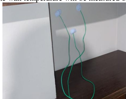
Fig.10. The placement of the triple sensor system on the wall.
