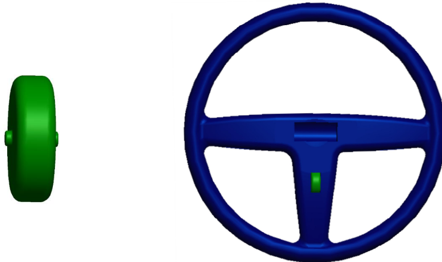
(VI-i-2~60) Control ring of level drive (VI-i-2~61) Control ring of level drive fixed on PNT engine steering wheel
