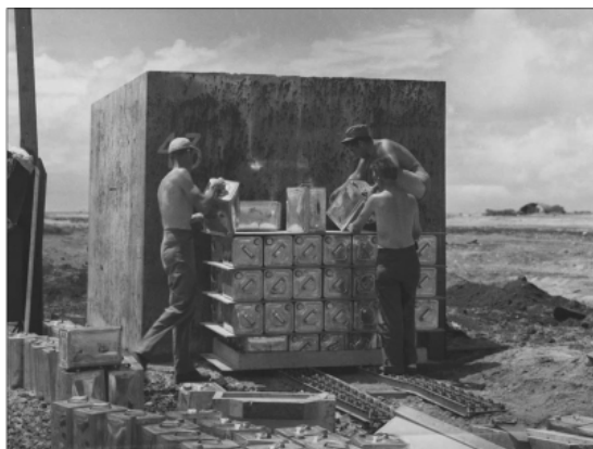
Figure 2: Empty 5 gallon cans being stacked against a blockhouse wall on Enewetak Atoll prior to an Operation Sandstone nuclear test in 1948. The degree to which the cans were crushed by the extreme pressures created by the explosion provided data on the blast's magnitude.
