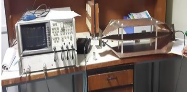
Fig. 2 Insertion loss test set up for Open TEM cell 1
