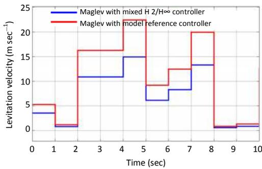
Fig. 8: Random response of train levitation velocity
