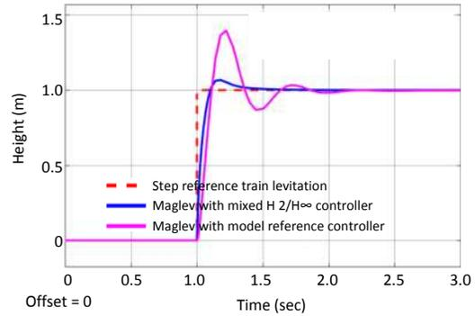
Fig. 4: Step response of train levitation height
