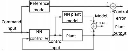
Fig. 3: Block diagram of the model reference controller
