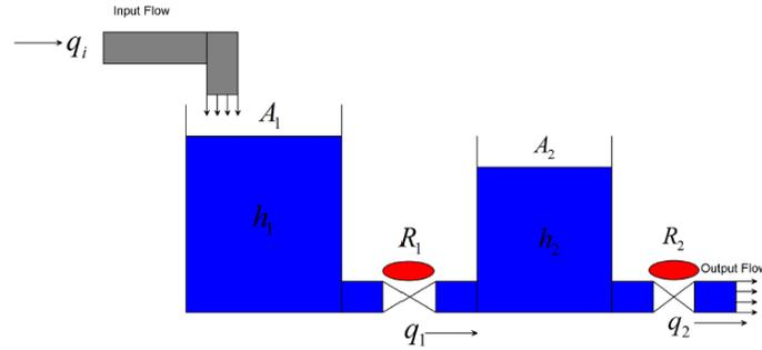
Figure 1 two-tank liquid-level control system
