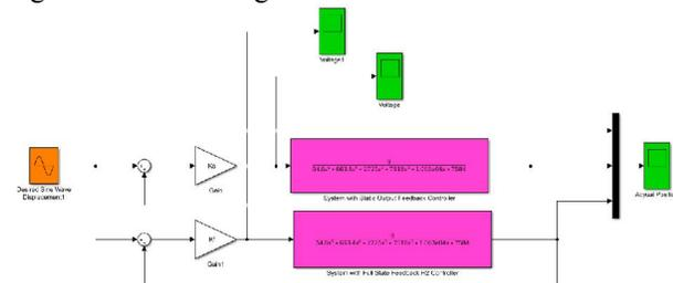
Figure 9 Simulink model of the cutting machine using static output feedback and full state feedback H<sub>2</sub> controllers using sine wave input desired position signal
