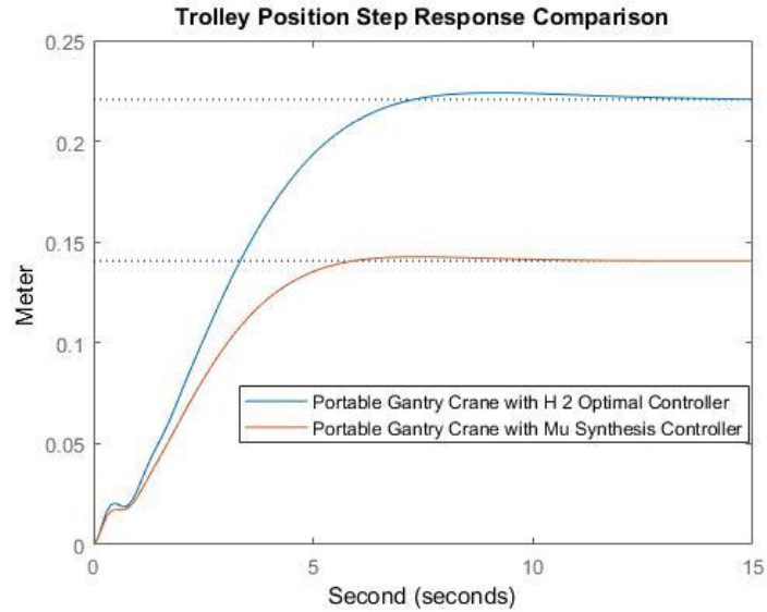
Figure 9 Comparison simulation result of the step response of the trolley position
