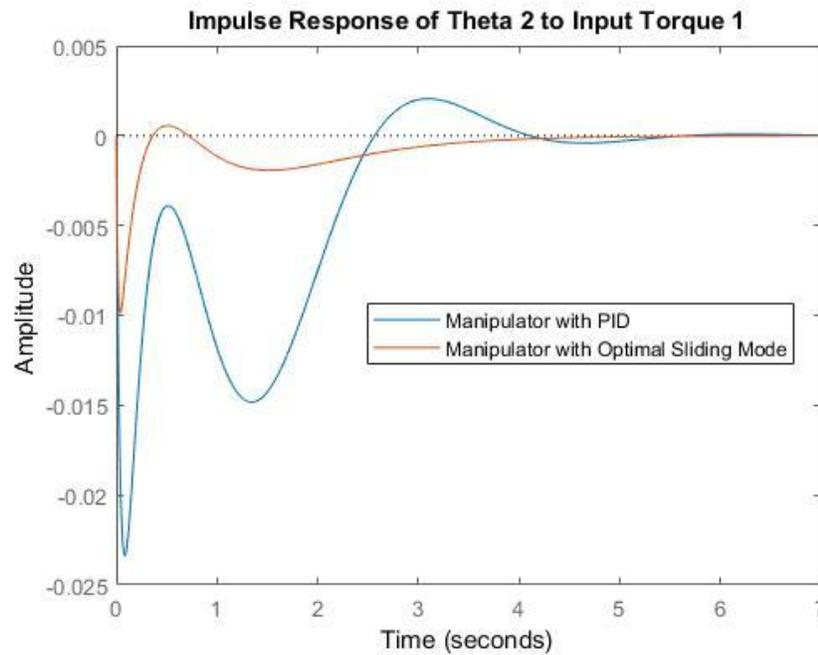
Figure 3 Impulse response of Theta 2 to Torque 1
