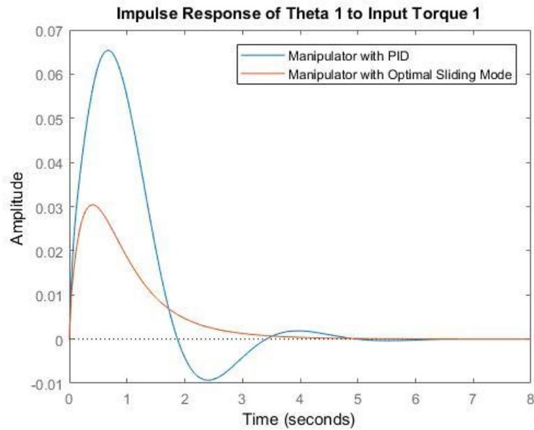
Figure 2 Impulse response of Theta 1 to Torque 1
