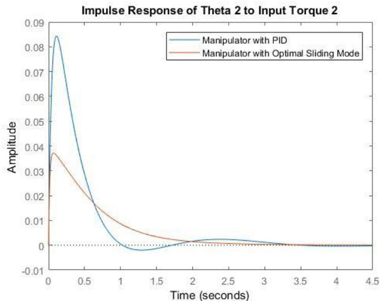
Figure 5 Impulse response of Theta 2 to Torque 2
