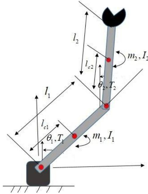
Figure 1 Vertically designed two link manipulator
