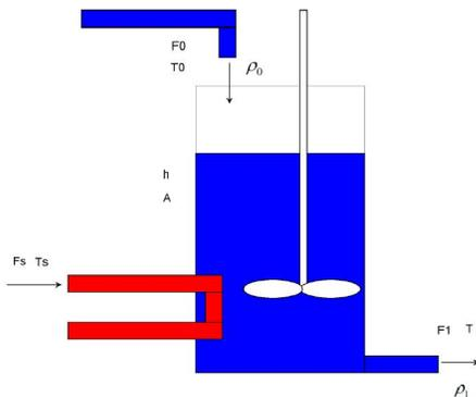
Figure 1 Stirred tank heater
