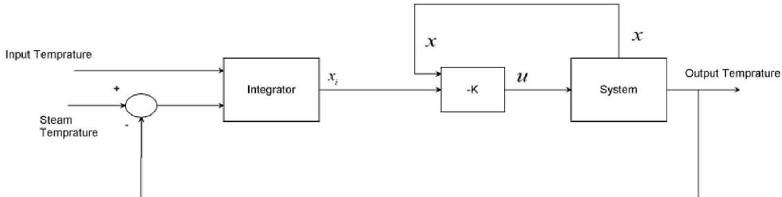
Figure 3 Block diagram of a stirred tank heater system with LQI controller
