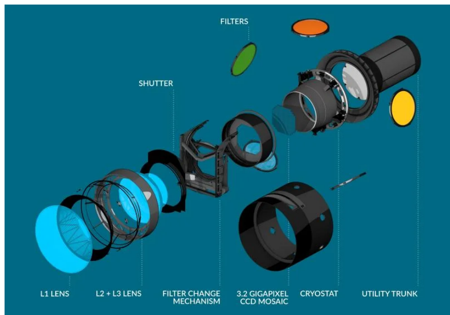
A digital diagram of the LSST Camera's main components. Credit: Chris Smith/SLAC National Accelerator Laboratory.
