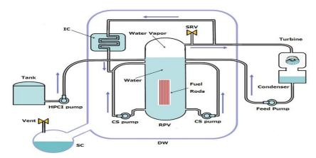
This is the inside structure of Unit1. Primary Containment Vessel (PCV) mentioned above is constituted of two parts: the main body called Drywell (DW), and the attached part called Suppression Chamber (SC). The core is located in DW, called Reactor Pressure Vessel (RPV). A blue-colored arrow "--" stands for a direction of a stream of fresh water.
