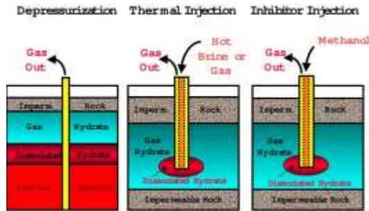
Figure 2: Hydrates production methods [14].
