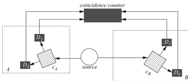
**Fig. 3** An experimental scenario testing for the non-separability of an entangled system of polarised photons. A source emits two entangled photons that travel to polarisers at  $c_A$  and  $c_B$ . In each of the regions  $A$  and  $B$ , one of the detectors  $D_0$  or  $D_1$  clicks, and this is recorded at a coincidence counter
