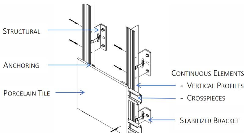
**Fig.1 Hidden anchoring system. Source [9]**
