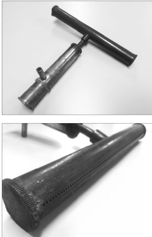
Figure 4: Smoking burner at Adelaide, made by Palmer (London). There are three of these in the Adelaide Heritage Collections: this one 22 cm wide, and two others 15 cm wide. The holes of all three are 1 mm in diameter, centres spaced 2 mm apart. The lower end is a capsule for benzol.
