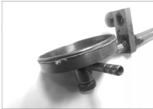
Figure 6: A tambour, made by Palmer, in the University of Adelaide Heritage Collections. Some fragments of the rubber membrane have survived natural degradation, as has the binding of thread that held it in place.
