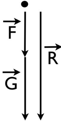
Figure 6: Resultant force of co-directional forces
