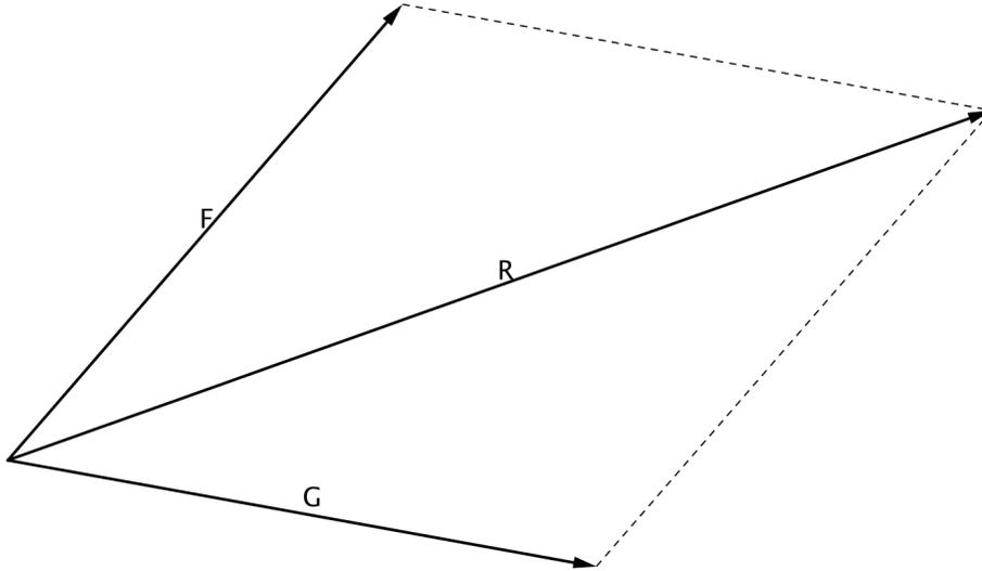
Figure 1: Parallelogram of forces
