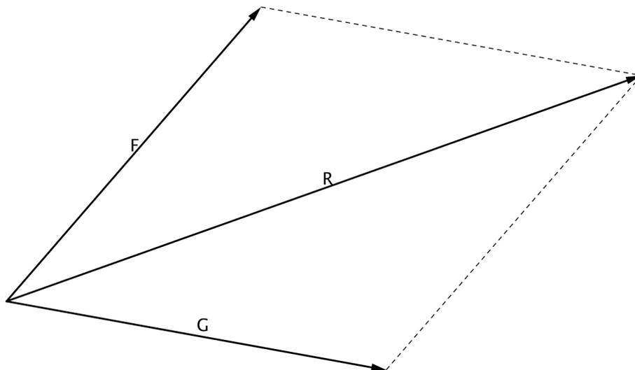
Figure 1: Parallelogram of forces
