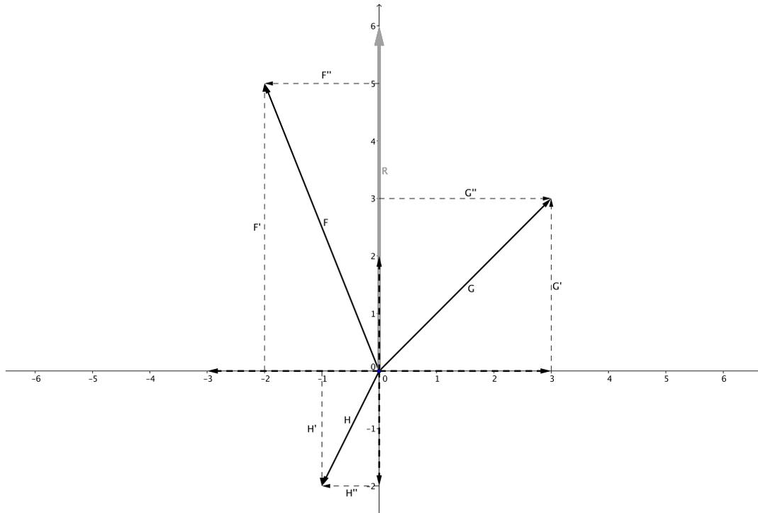
Figure 9: Composition of three non-collinear forces
