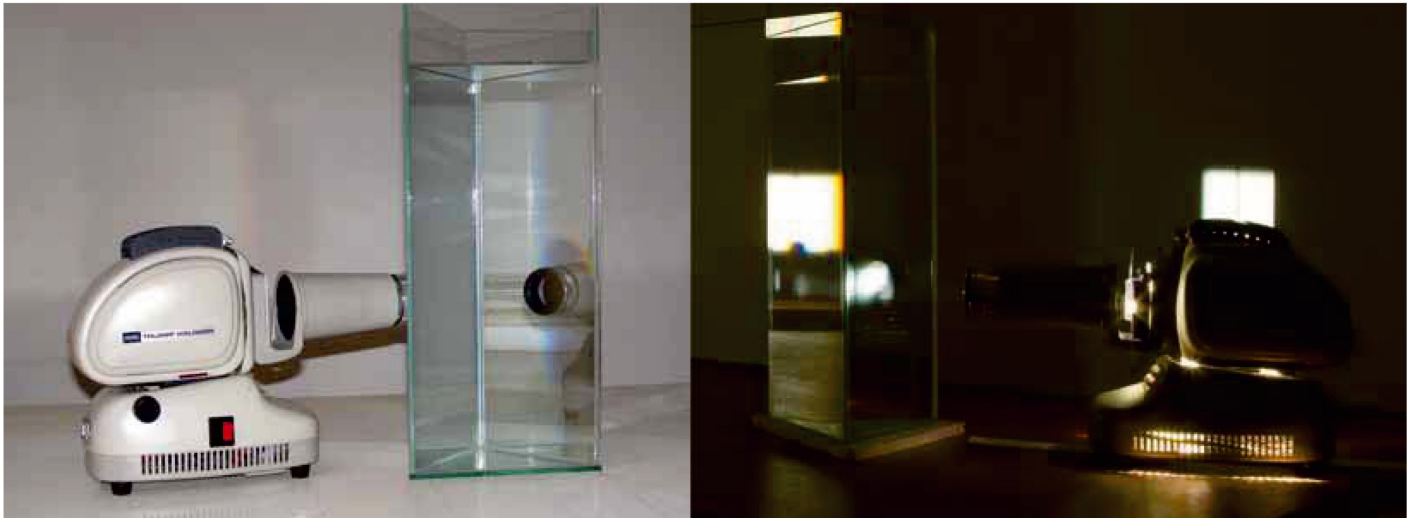
Fig 2 Projector and water prism in Nussbaumer's dark chamber [I.N. 2009]. The prism is not illuminated by the sun in Nussbaumer's version of Newton's experiment (Fig. 1), but by the light from a slide projector (that projects the image of a slide with a gap on it). The light from the projector's bulb is weaker than the sun's, but it hardly differs with respect to its composition.
