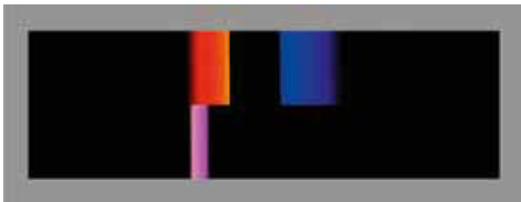
Fig 9 Photograph of the Viennese purple synthesis [J.N. 2009]. The top of the figure shows a picture of the Newtonian spectrum with its green centre cut away by Nussbaumer. The bottom shows a picture of this fragmented spectrum taken by the camera through the refracting prism. All the colours of the Newtonian spectrum (except green) converge and mix into purple, which is green's complement.
