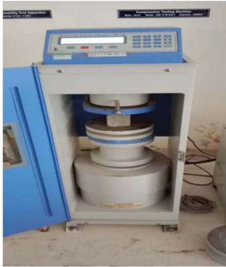
Fig. 9: Test set up for compressive strength
