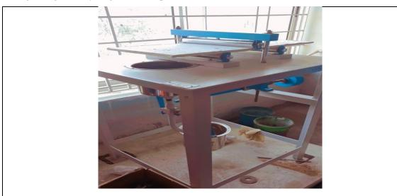
Fig. 12: Flexural Strength Testing Machine
