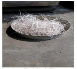
Fig. 4: Plastic Fibre
