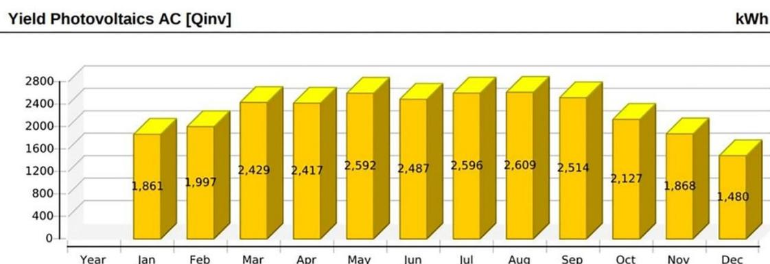
**Figure 5.** The energy produced by photovoltaic modules monthly
