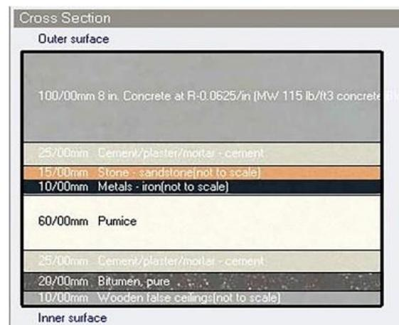
Figure 1. Details of the composite roof layers in DesignBuilder software
