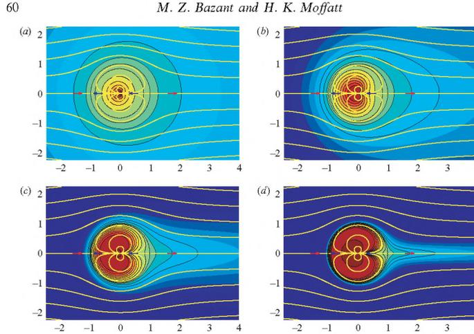
FIGURE 3. Steady vortex avenues confined by transverse flow with a dipole source inside and a uniform background flow outside (a dipole at  $\infty$ ). These transverse jets exhibit a non-trivial dependence on the Reynolds number with a transition from ‘clouds’ to ‘wakes’ of vorticity: (a)  $Re = 0.1$ , (b)  $Re = 1$ , (c)  $Re = 10$ , (d)  $Re = 100$ .
