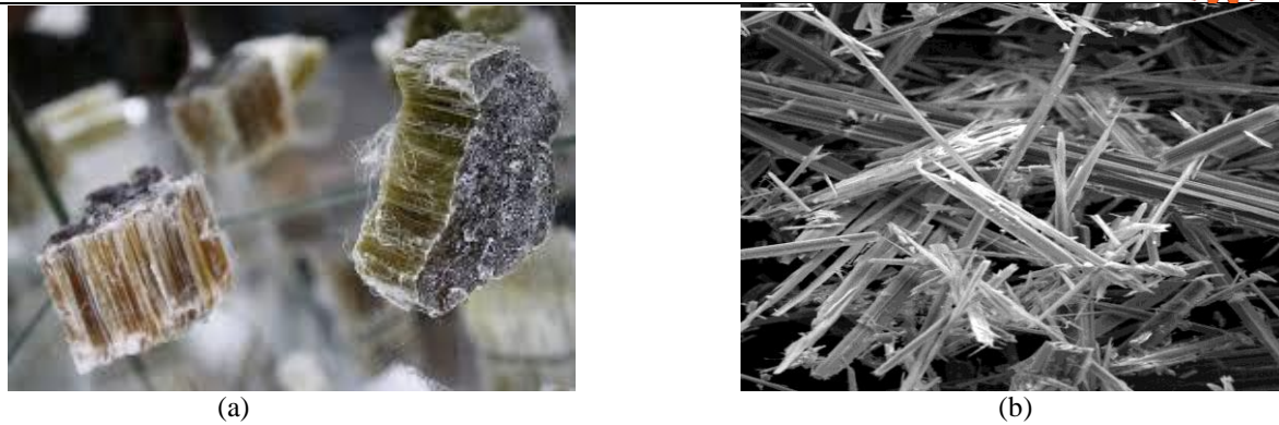
Figure 1. Asbestos Minerals (a) and how its look Asbestos in microscope (b)
