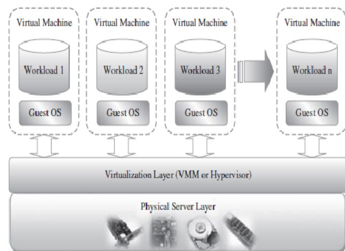
Fig. 1: Layered Virtualization architecture.
