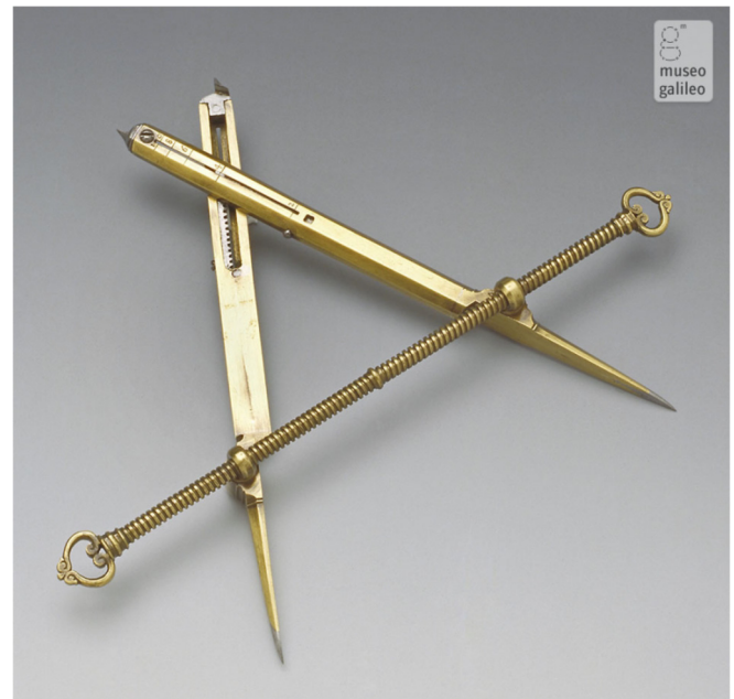
Fig. 1. An example of a reduction compass from the Medici Collections (Museo Galileo, Florence – Photography by Franca Principe).
