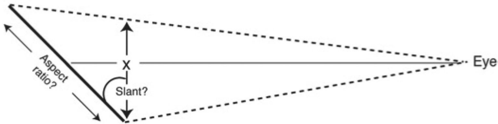
Figure 5 If x is the aspect ratio of the image projected on to a 2D plane from a 3D surface, then one can infer the aspect ratio of the 3D surface ( A ) given the slant of the 3D surface ( R ). That is, A = x(\cos(S)) . Image from Geisler and Kersten (2002).
