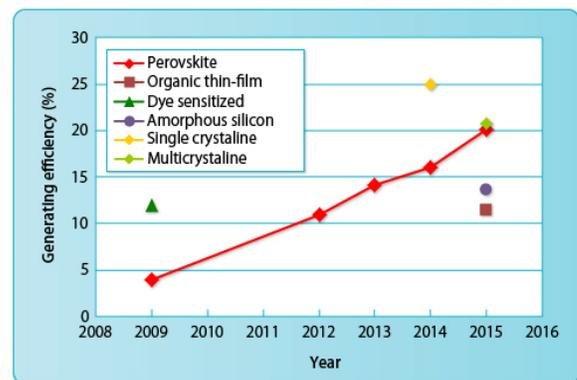
Fig. 2. Trends in maximum conversion efficiency for solar cells at the research stage
