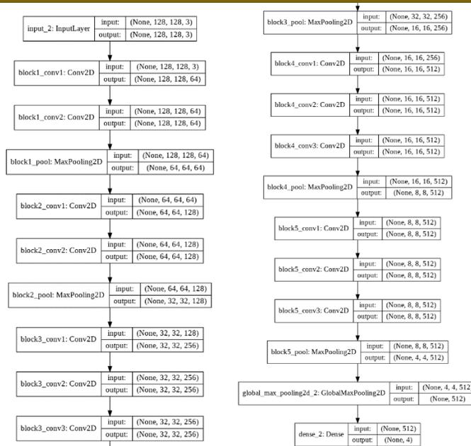
Figure 5 Architecture of VGG 16 model
