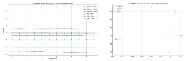
Responsiveness: The delay between gesture input and vehicle response was measured to be less than 200ms, so the system was very responsive.
