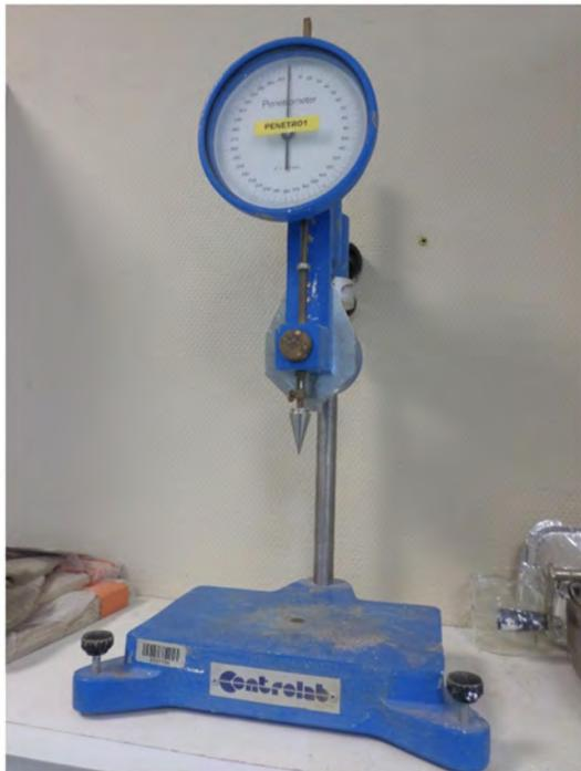
Fig. 13. Laboratory penetration cone.
