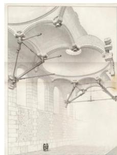
Eugène Viollet-le-Duc. Design for a brick vault supported by iron, replacing the need for an external stone buttress. From: *Entretiens sur l'Architecture* (Paris, 1863).
