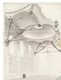
Eugène Viollet-le-Duc. Design for a brick vault supported by iron, replacing the need for an external stone buttress. From: *Entretiens sur l'Architecture* (Paris, 1863).
