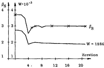
Figure 4. Iteration history for failure defined at mechanism level. x indicates identification of significant failure modes. The NLPQL algorithm is used.
