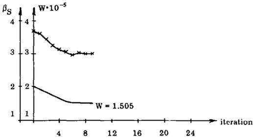
Figure 7. Iteration history for failure defined at mechanism level. x indicates identification of significant failure modes. The simple optimization algorithm in section 4 is used.
