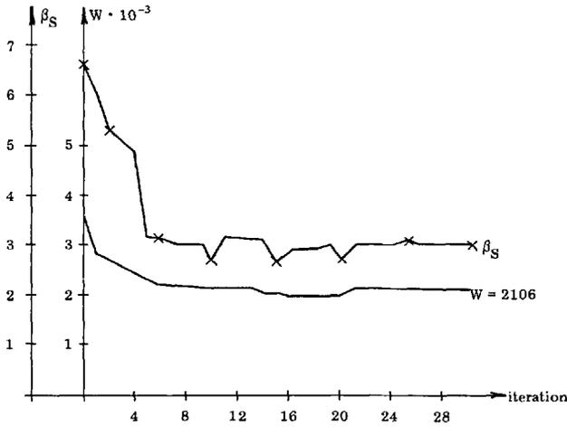
Figure 3. Iteration history for failure defined at level 2. x indicates identification of significant failure modes.
