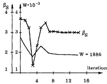
Figure 5. Iteration history for failure defined at mechanism level. x indicates identification of significant failure modes. The simple optimization algorithm in section 4 is used.
