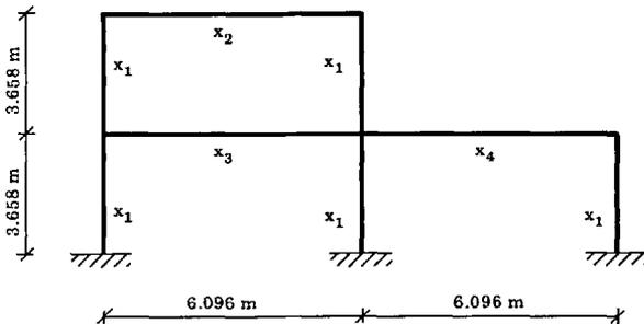
Figure 2. Geometry and optimization variables.
