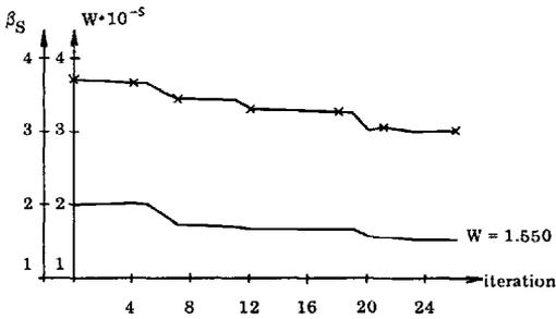
Figure 8. Iteration history for failure defined at mechanism level. x indicates identification of significant failure modes. The NLPQL algorithm is used.
