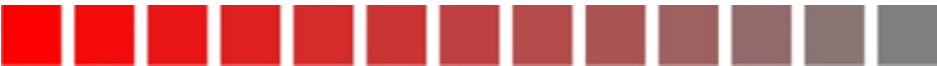
Fig. 11.3 Samples of colours with the same hue and brightness, but with different saturation.
