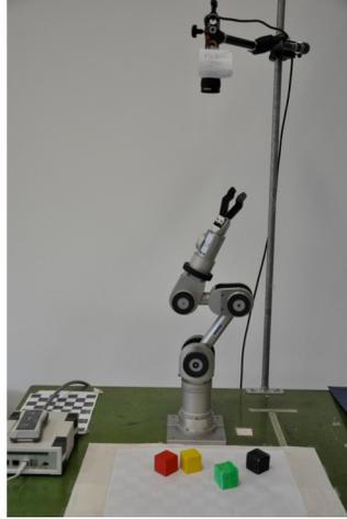
**Figure 2.** The Katana robot arm. Source: Ngo 2012.
